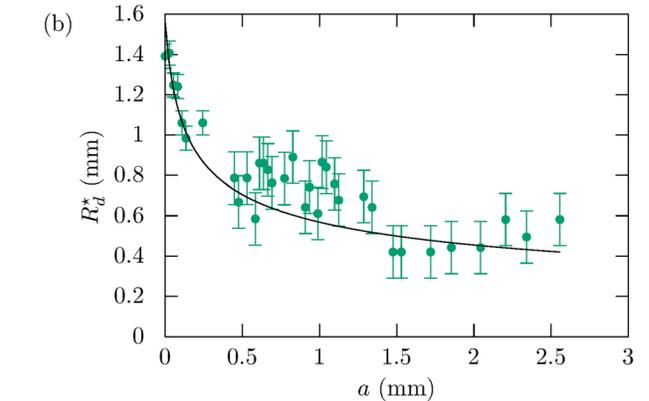
FIG. 3. Drop motion on a horizontal vibrating fiber. (a) Time-lapse image of a water drop placed on a node and an antinode. The plot shows the displacement imposed at the upper end of the fiber. The drop volume is 5  $\mu\text{l}$  and the oscillation amplitude and frequency are 0.34 mm and  $f = 140$  Hz, respectively. (b) Critical radius after which the drop detaches from the fiber versus the local amplitude  $a$  of the fiber. The solid line is Eq. (6).
