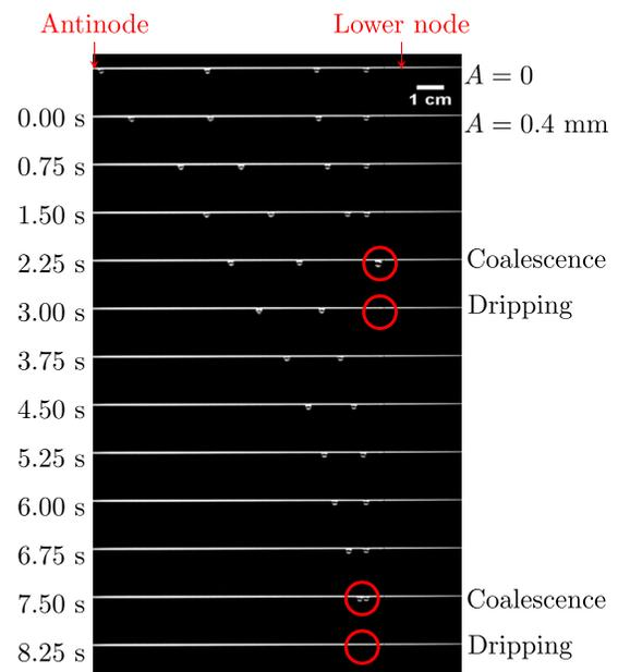
FIG. 5. Illustration of multiple drop manipulation on an inclined fiber. Initially, evenly spaced drops are placed on the fiber. As vibrations start, the drops slide, coalesce near the node, and fall off the fiber. For this experiment,  $\theta = 16^\circ$ ,  $f = 100$  Hz,  $A = 0.4$  mm, and the drop volume is  $5 \mu\text{l}$ . (Multimedia view) [URL: <http://dx.doi.org/10.1063/1.4935251.1>]
