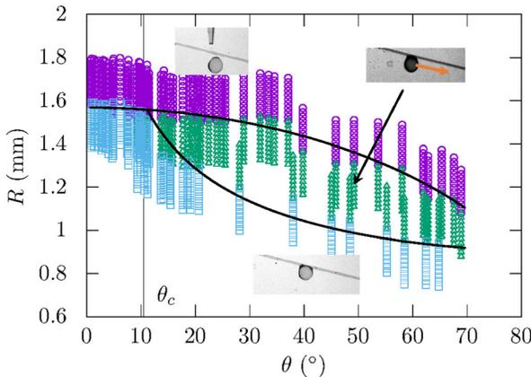
FIG. 2. Phase diagram of drop behavior on a static fiber as a function of the drop radius  $R$  and the fiber inclination angle  $\theta$ . Three distinct domains are observed: static ( $\square$ ), sliding ( $\triangle$ ), and dripping ( $\circ$ ). The upper and lower solid lines represent Eqs. (2) and (4), respectively. In Eq. (4), we used  $F_f^{max} = 3 \times 10^{-5}$  N. The angle  $\theta_c = 11^\circ$  denotes the critical angle above which the three domains can be observed.
