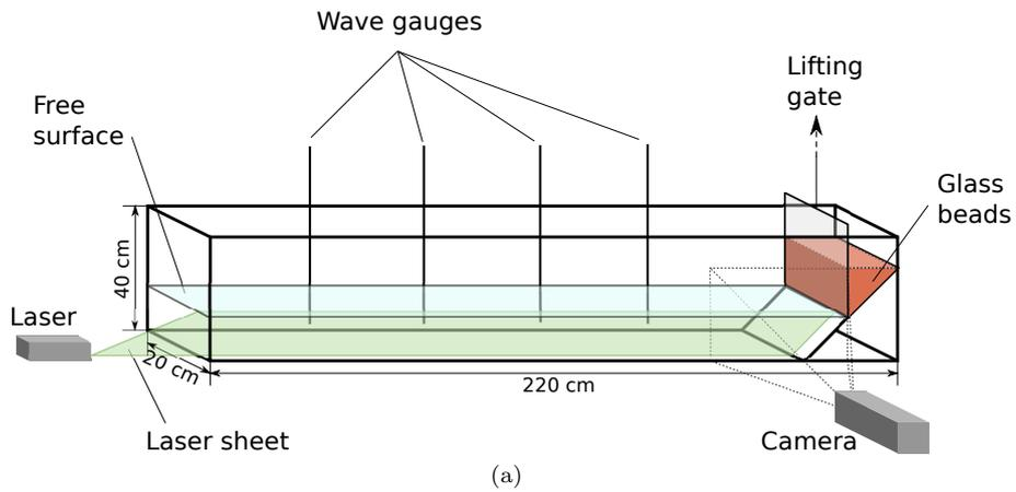
**Fig. 1** Schematic view of the experimental set-up
