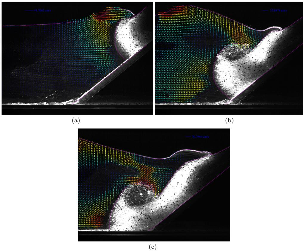
**Fig. 2** Sequence of snapshots showing the granular collapse and the generated wave for a slope angle of  $45^\circ$  and 3.00 kg of beads. At time (a)  $t = 230$  ms, (b)  $t = 410$  ms and (c)  $t = 520$  ms. PIV field are also represented.
