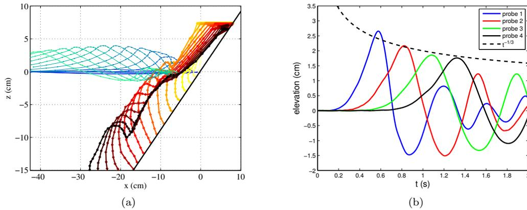
**Fig. 3** (a) Evolution of the free surface and the granular flow during the collapse and (b) elevation of the free surface at each probe for the parameters used in Fig. 2.
